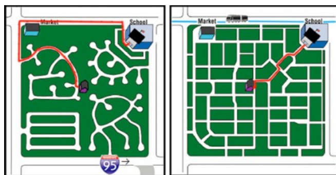
Figure 10: Non-Uniform, Disconnected Layout vs. Uniform, Connected Layout
