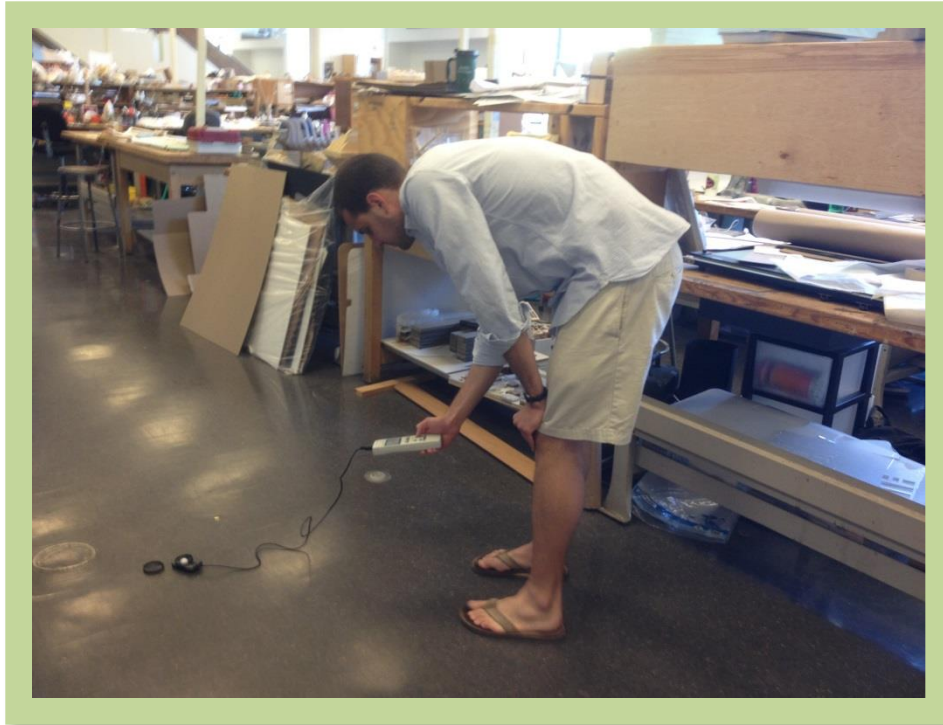
The three images above show daytime data collection of the light levels using the light meter (Photos by Morgan Stackman)
