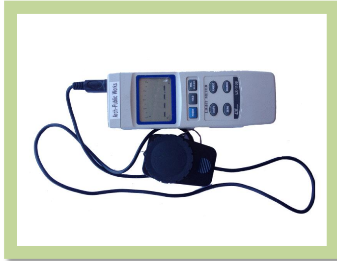
The picture above shows the light meter used during data collection to monitor the ambient light levels in the studio areas of Campbell Hall. All light levels were recorded in foot candles, and some important features include the range button, which allows for more accurate measurements, and the zero button which allows for the instrument to record consistent data.
