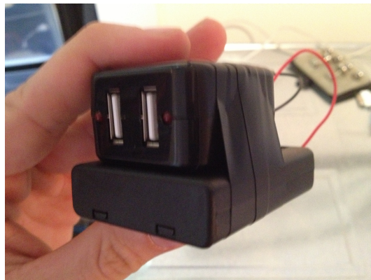
Figure 3: Battery Power Source and USB Charger for Turbine
