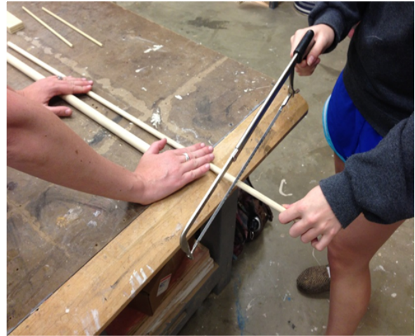
Figure 5: Cutting the dowel
